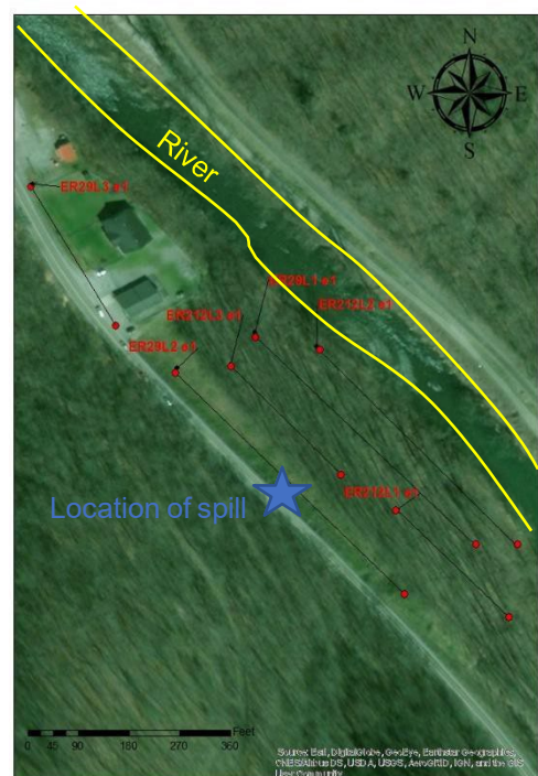
Figure 1. Map showing the layout of the ER surveys trending SE to NW. These types of maps are constructed, geolocated and projected using ArcGIS and sent to our clients. The blue star indicates the spill site and the river is outlined in yellow.
